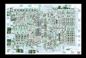
2,300 Transistors 10,000 Nanometers 740 KHz (.00074 GHz) ≈ \$1 (1968) **2018: Intel Core i9-8950HK**
